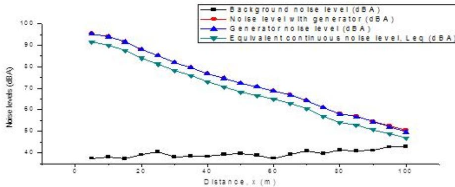
Figure. 1: A 500 kVA power generator noise levels against distance
