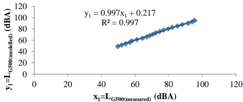
Figure 4: Comparison of modeled noise levels,  $L_{G500(\text{modelled})}$  and measured noise levels,  $L_{G500(\text{measured})}$  of a 500 kVA power generator
