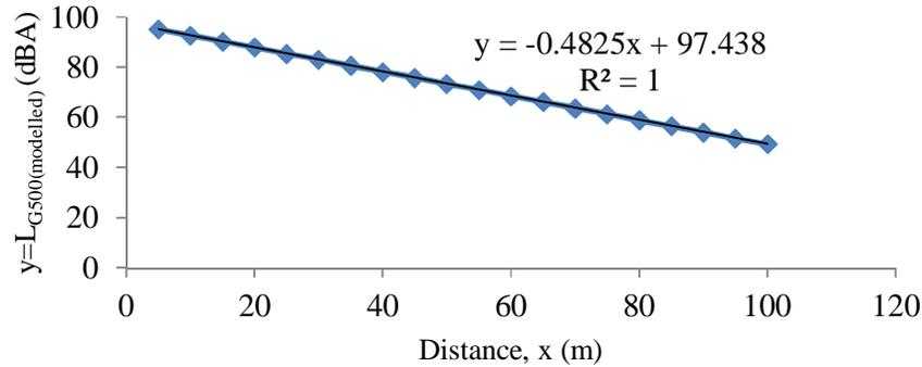
Figure 3: The characteristics of the 500 kVA power generator modeled noise level
