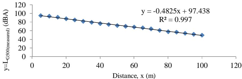
Figure 2: The characteristics of the 500 kVA power generator measured noise level
