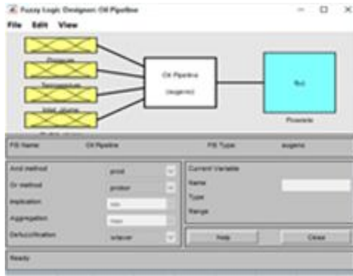
Figure 2a: Oil Pipeline ANFIS Structure
