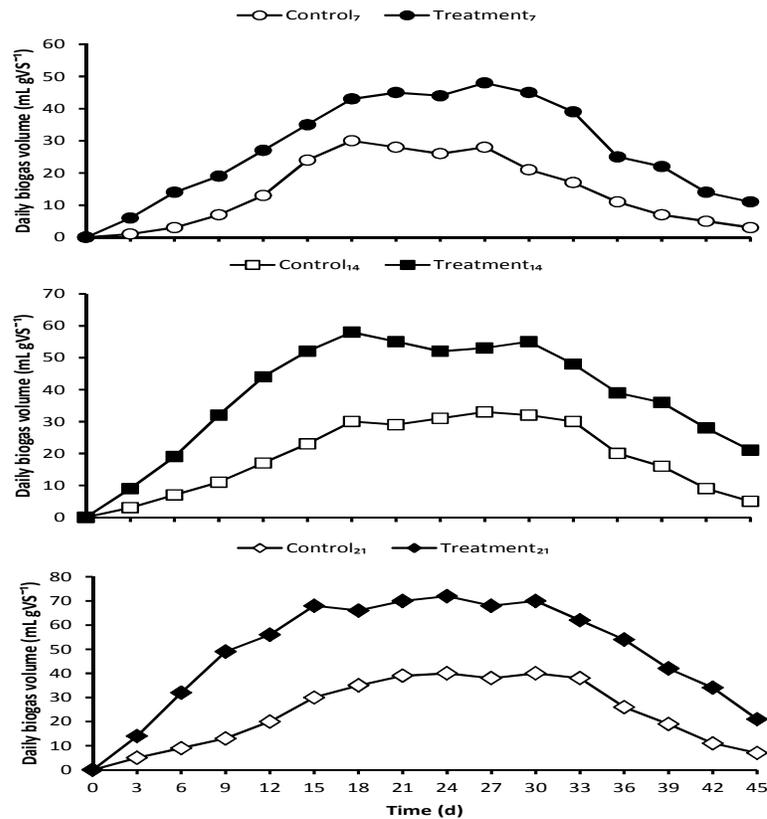
Figure 1: Influence of cassava mill effluent pretreated rice husk lignocellulosic biomass on biogas production.
