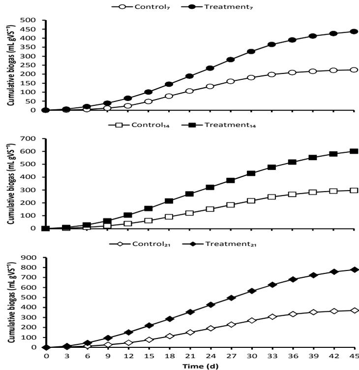
Figure 2: Cumulative biogas production from rice husk lignocellulosic biomass pretreated with cassava mill effluent.
