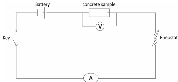
Figure 1: Circuit diagram showing the experimental set-up
