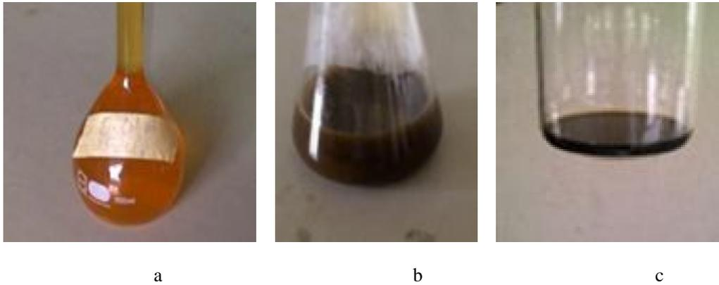
Figure 2: Vials containing samples of (a) ferric chloride, (b) *Kola acuminata* extract, (c) iron nanoparticles
