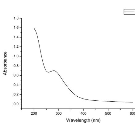
Figure 3: UV-Vis spectrum for the prepared FeNPs
