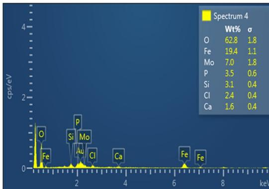
Figure 5: EDS spectrum of the iron nanoparticles
