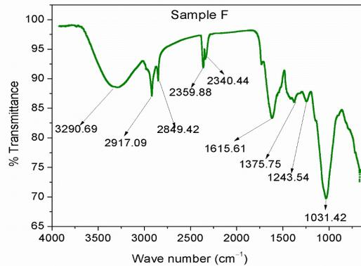
Figure 4: FTIR spectrum of the FeNPs
