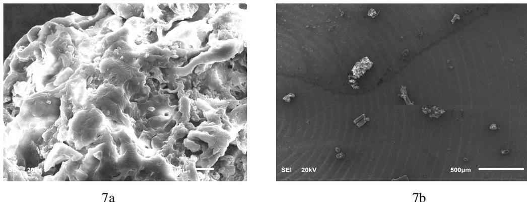
Figure 7. SEM images of the synthesized iron nanoparticles: a, 10µm; b, 500µm
