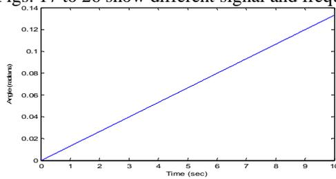
Fig. 17: Open loop step response of dc motor
