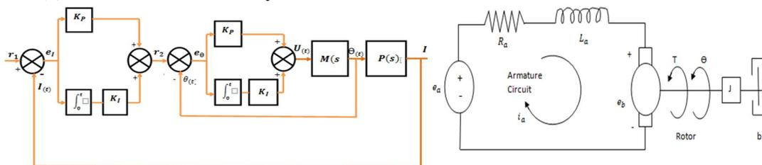
Fig.1a. Cascade control system block diagram of solar tracker
