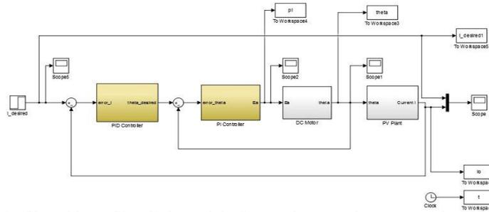
Figure 16: Closed loop Simulink model of cascade control system of the solar tracker
