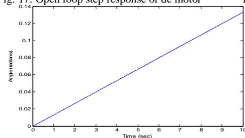
Fig. 19: Open loop step response of dc motor coupled to PV system
