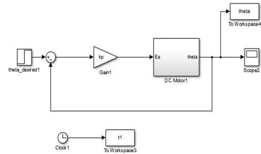
Fig. 13: Simulink model of Kp on dc motor system
