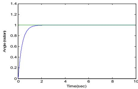
Fig. 23: Output closed loop response of dc motor with controller
