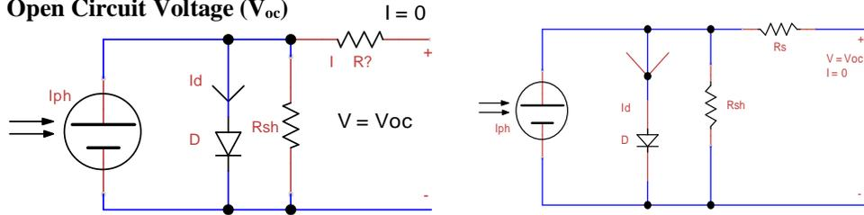
Fig. 6: Complete Photovoltaic Cell Model Fig. 7: Equivalent Photovoltaic cell model showing open circuit voltage
