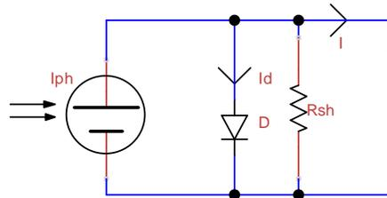
Fig. 4: Series resistance configured photovoltaic cell
