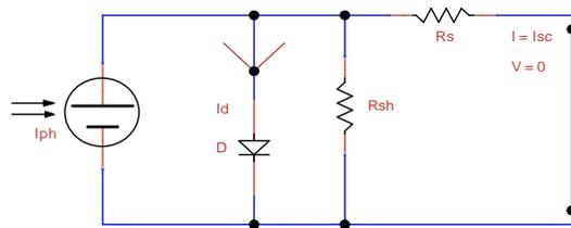
Figure 8: Equivalent photovoltaic Cell Model with Output short
