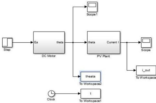
Fig. 12: Simulink diagram of open loop process plant
