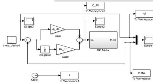
Fig. 14: Closed loop Simulink model of dc motor with controller
