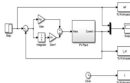
Figure 15: Closed loop Simulink model of PV with PI controller
