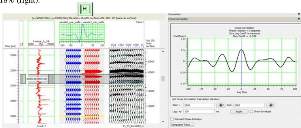
Figure 14: Re-extracted well option wavelet used for well correlation by stretching and squeezing technique leading to the crosscorrelation plot of time shift 0ms and correlation coefficient of 53% (right).
