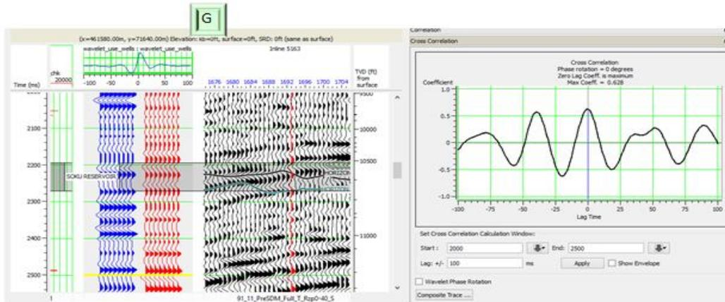
Figure 12: Re-extracted well option wavelet used for well correlation by stretching and squeezing technique leading to the crosscorrelation plot of time shift 0ms and correlation coefficient of >60% (right)
