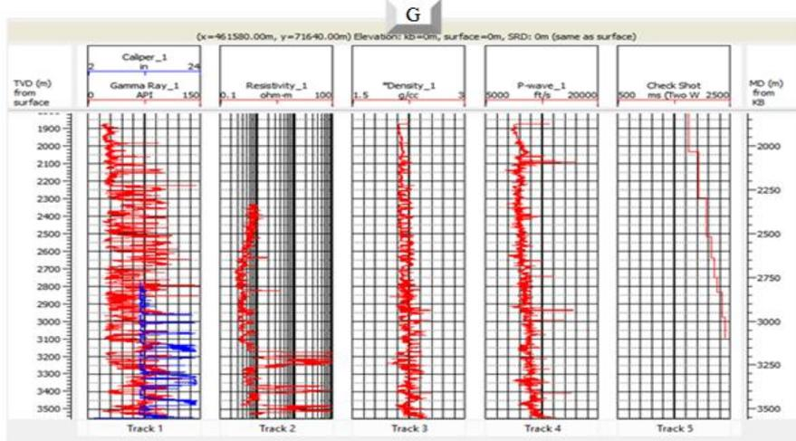
Figure 2: Suite of imported logs for Well G showing log signatures of Gamma ray, Resistivity, Density and P-wave.
