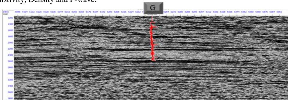
Figure 4: Inline and Crossline baseline seismic section  $\eta$  field between 1200-3800ms showing P-wave log at Well G.
