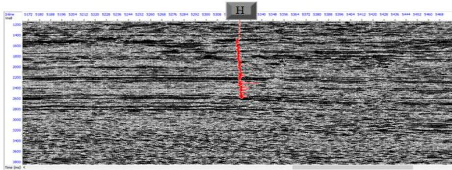
Figure 5: Inline and Crossline baseline seismic section  $\eta$  field between 1200-3800ms showing P-wave log at Well H.
