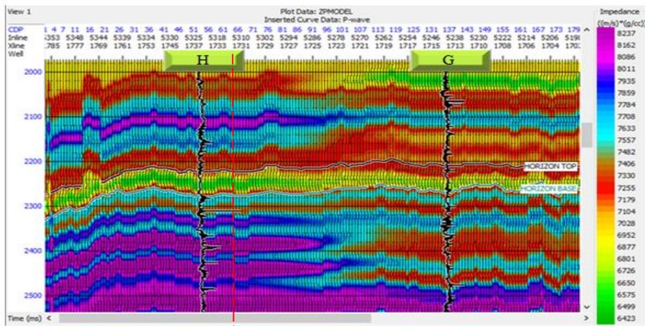
Figure 16: Inline/Xline arbitrary view of seismic section superimposed with colour section (initial model P-impedance) between 2000-2500ms showing P-wave log plot at Well G and Well H. Picked Horizons across the top and base of Reservoir expected where low P-Impedance log is bounded by low section of initial model
