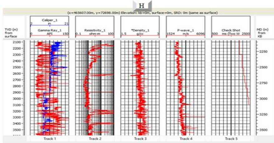
Figure 3: Suite of imported logs for Well H showing log signatures of Caliper, Gamma ray, Resistivity, Density and P-wave.
