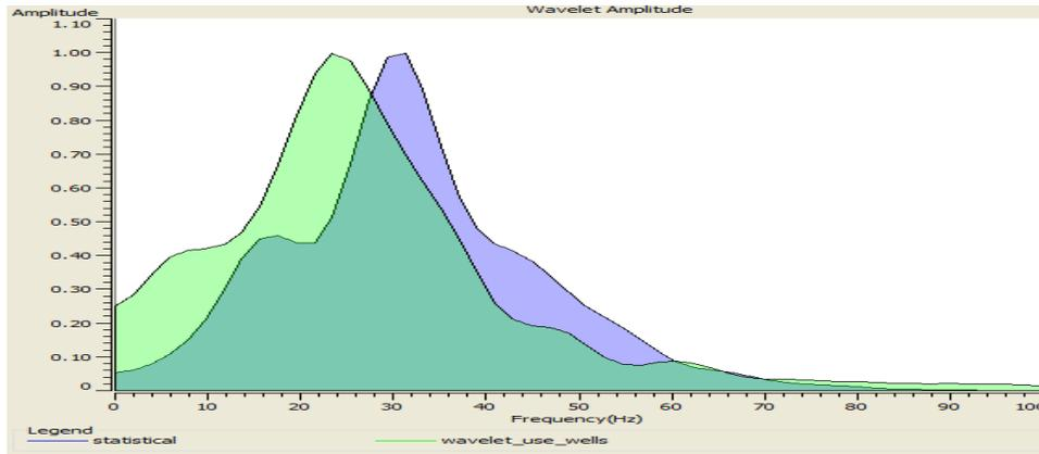
Figure 15: Amplitude spectrum of statistical (blue) and re-extracted (green) wavelets
