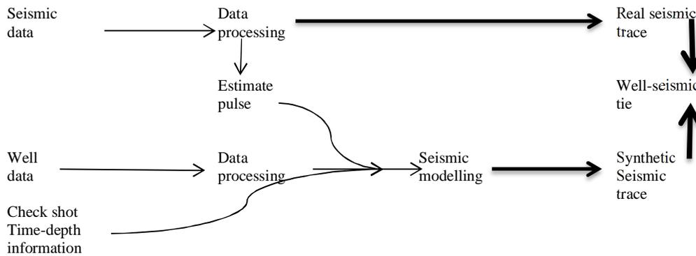
Figure 7: Well-to-Seismic Tie workflow
