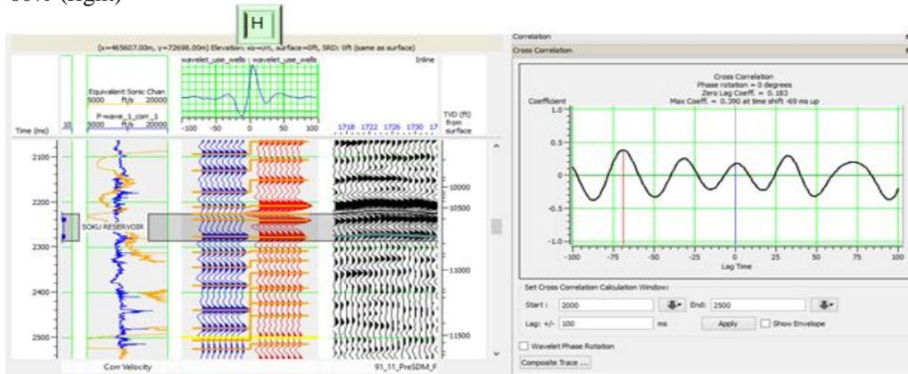
Figure 13: Statistically extracted wavelet used for well correlation by stretching and squeezing technique resulting in crosscorrelation plot of time shift -69ms up and correlation coefficient of <18% (right).
