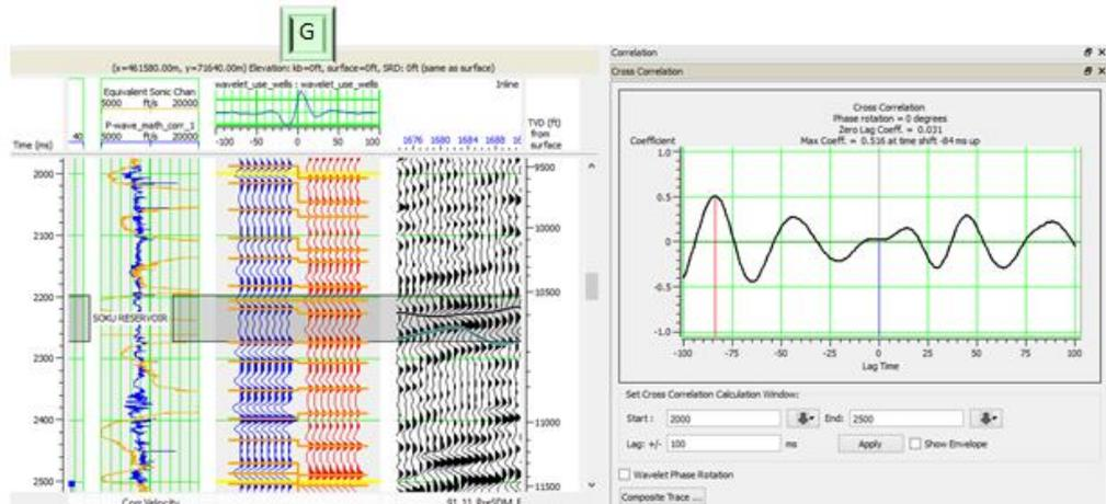
Figure 11: Statistically extracted wavelet used for well correlation by stretching and squeezing technique resulting in crosscorrelation plot of time shift -84ms up with correlation coefficient of <51% (right).
