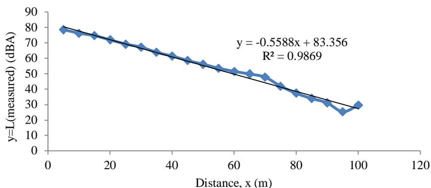
Fig. 2: The characteristics of the business centre measured noise level
