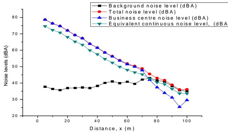
Fig. 1: A plot of the business centre with a maximum noise level of (83.35±0.91) dBA against distance
