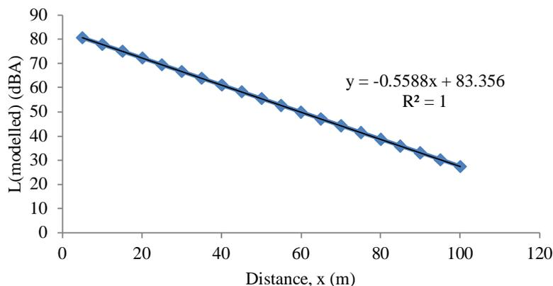
Fig. 3: The characteristics of business centre modelled noise level
