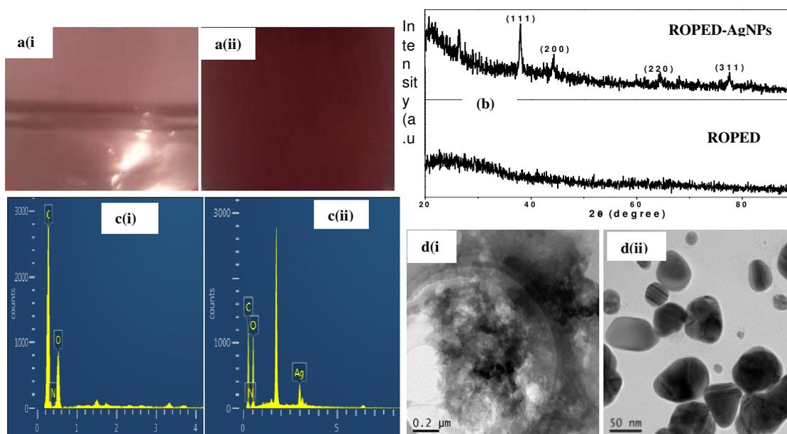
Figure 2: (a) Colour of (i) ROPED and (ii) ROPED-AgNPs (ii) XRD spectra of ROPED and ROPED-AgNPs (c) EDS spectra of (i) ROPED and (ii) ROPED-AgNPs and (d) TEM images of (i) ROPED and (ii) ROPED-AgNPs
