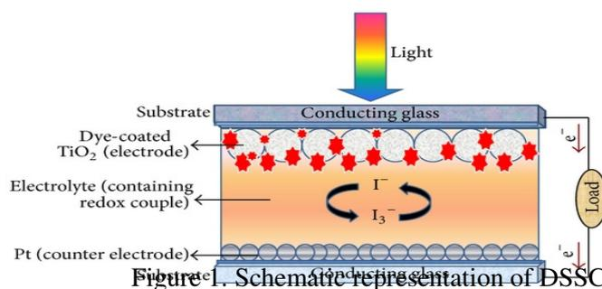
Figure 1. Schematic representation of DSSC
