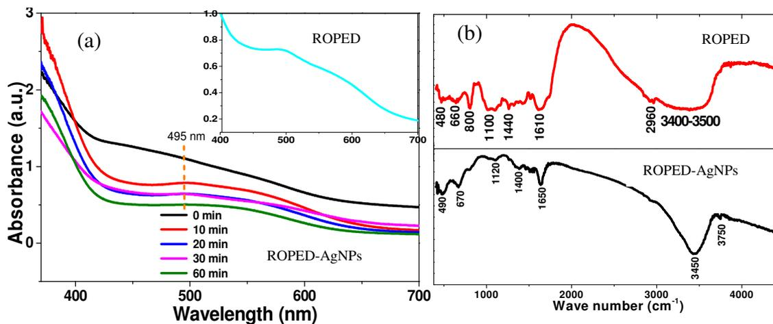
Figure 3: (a) UV-Vis Spectra of ROPED and ROPED-AgNPs at various time during development and (b) FTIR spectra of ROPED and ROPED-AgNPs.
