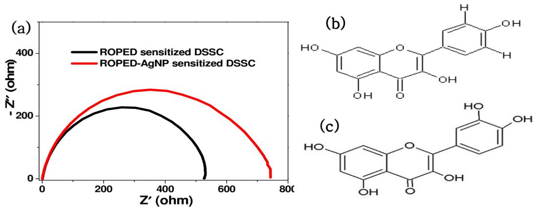
Figure 4:(a) Nyquist plots obtained from EIS study of ROPED sensitized and ROPED-AgNPs sensitized DSSC (b) molecular structure of kaemferol and (c) molecular structure of quercetin.
