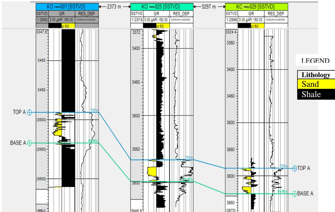
Figure 4: Delineation of reservoir tops on the well section.
