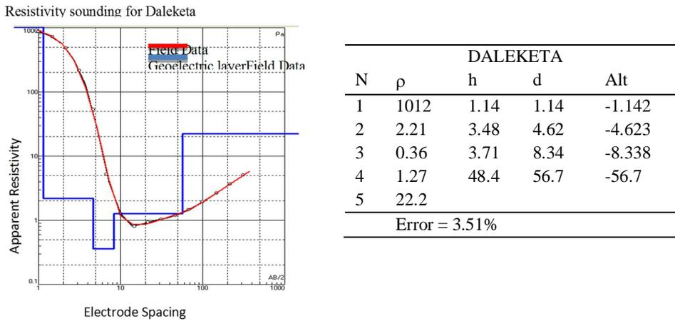
Figure 5: VES curve and layers resistivity for Daleketa
