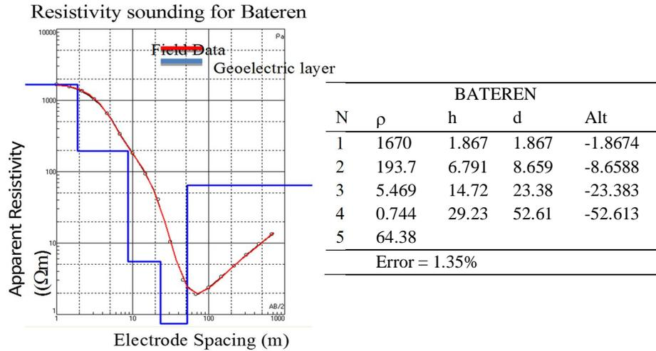
Figure 4: VES curve and layers resistivity for Bateren.
