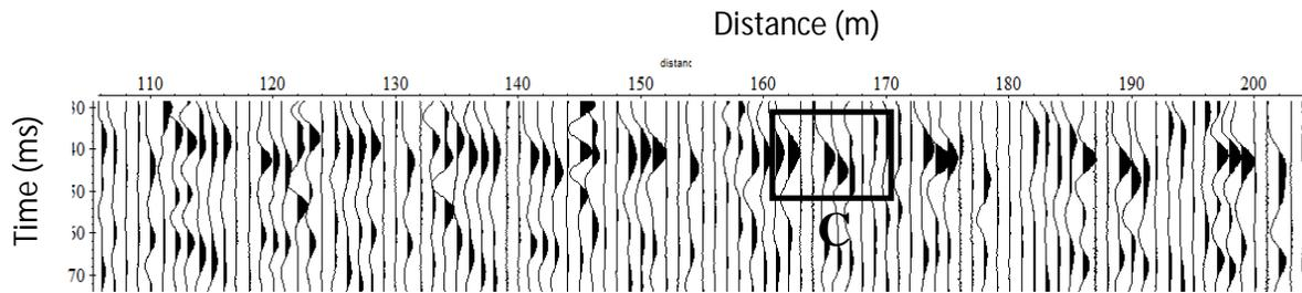
Figure 7: Seismic profile, sorted into CMP Traces for AVO analysis
