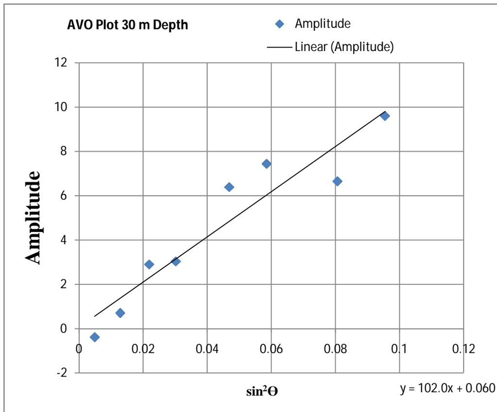
Figure 9: Amplitudes from each time sample of a gather C, figure 8 plotted against the squared sine of the angle-of-incidence.
