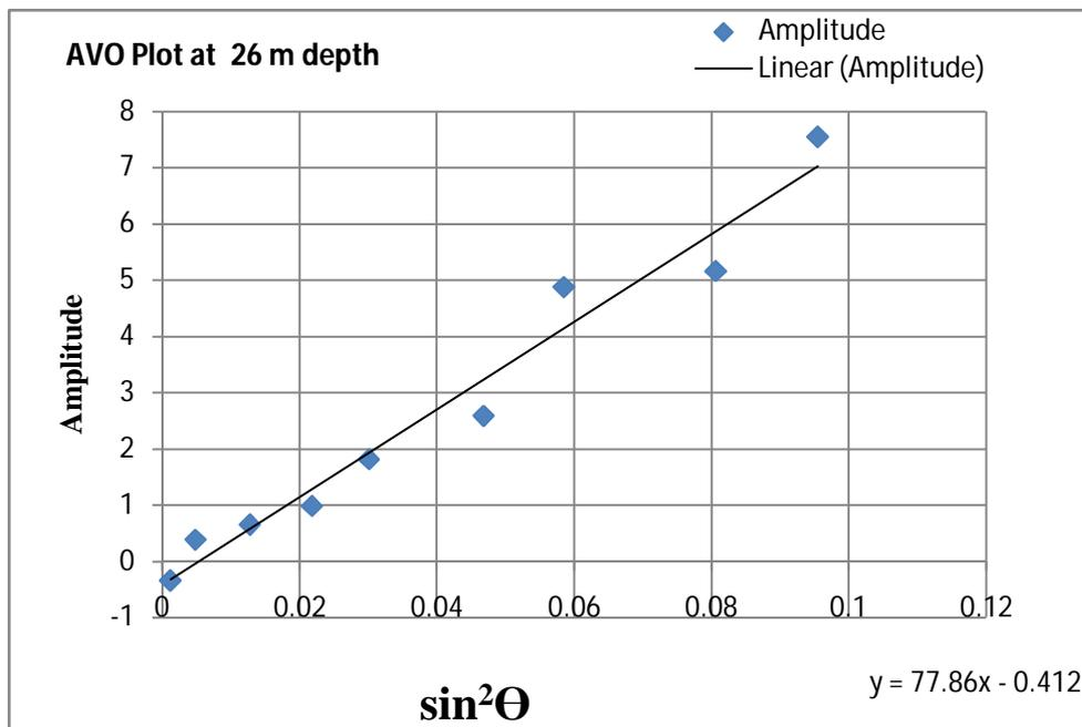
Figure 6: Amplitudes from each time sample of a gather B, figure 5 plotted against the squared sine of the angle-of-incidence.
