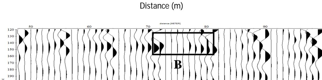
Figure 4: Seismic profile, sorted into CMP Traces for AVO analysis
