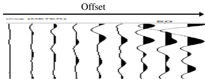
Figure 5: AVO Signature extracted from figure 4, sorted into CMP Traces
