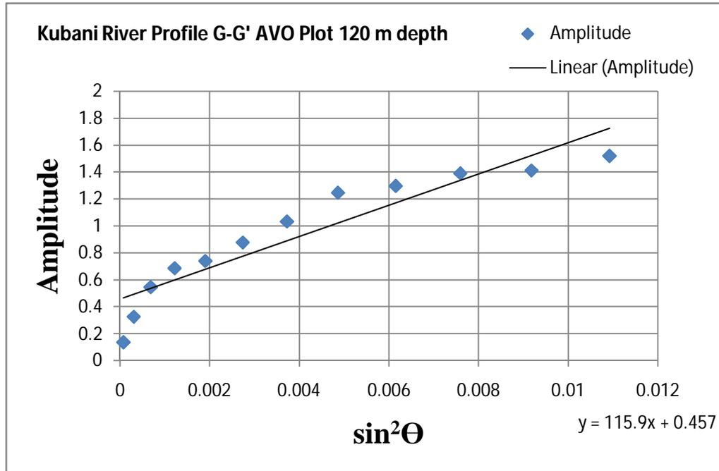
Figure 3: Amplitudes from each time sample of a gather A at 120 m depth, vs squared sine of the angle-of-incidence.
