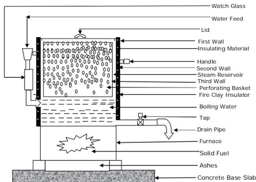
**FIG. 4: Structure of Steam Rice Par-boiler**
