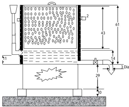
**Figure 3 Cross sectional Layout of Rice Steam Parboiler (All dimensions in cm)**
