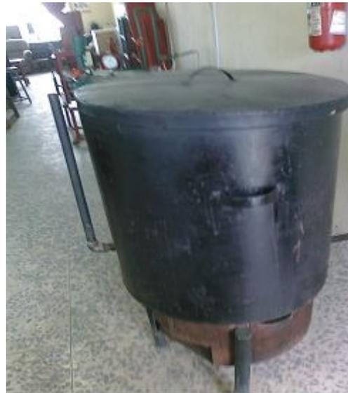
**Fig. 5: Locally Fabricated Steam Rice Par-Boiler**
