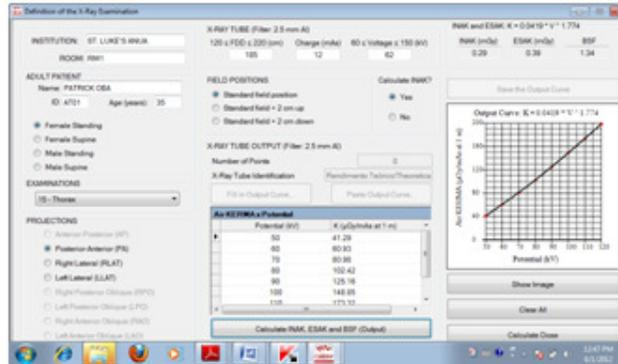
Fig.4: Theoretical output curve, the INAK, the ESK and the back-scatter factor (BSF)
