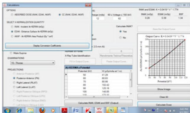
Fig.8: Selection of output mode for results: Conversion coefficients between organ and tissue absorbed doses and ESAC.
