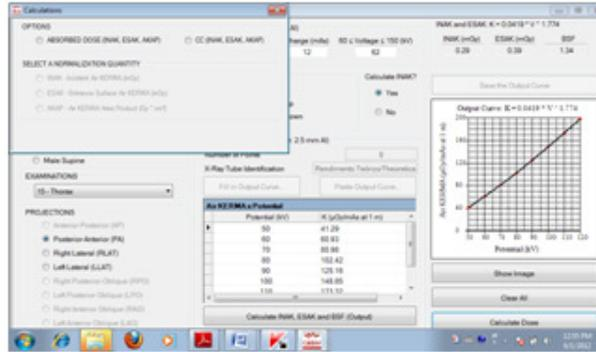
Fig. 6: Selection of output mode for results: Organ and tissue absorbed dose based on INAK
