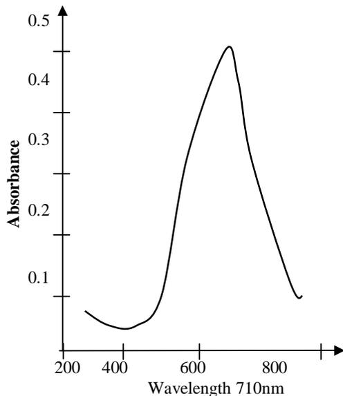
Fig 1: Spectrum of the blue complex formed from the reaction of  $5\mu\text{g/ml}$  of DHA, 2ml of 0.2% Ferric chloride and 2ml of 0.2% of Potassium Ferricyanide
