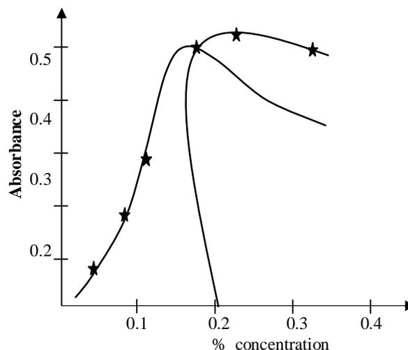
Fig 2: Effect of Ferric chloride and Ferricyanide concentration on Absorbance of the blue complex measured at  $710\text{nm}$ , of  $5\mu\text{g/ml}$  of DHA at  $45^\circ\text{C}$ .
