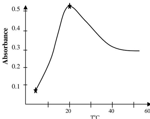
Fig. 4: Effect of Temperature on the absorbance of the blue complex at 710nm, when 5µg/ml of DHA reacted with 2ml of 0.2% FeCl<sub>3</sub> and 2ml of 0.2% Ferric chloride.
