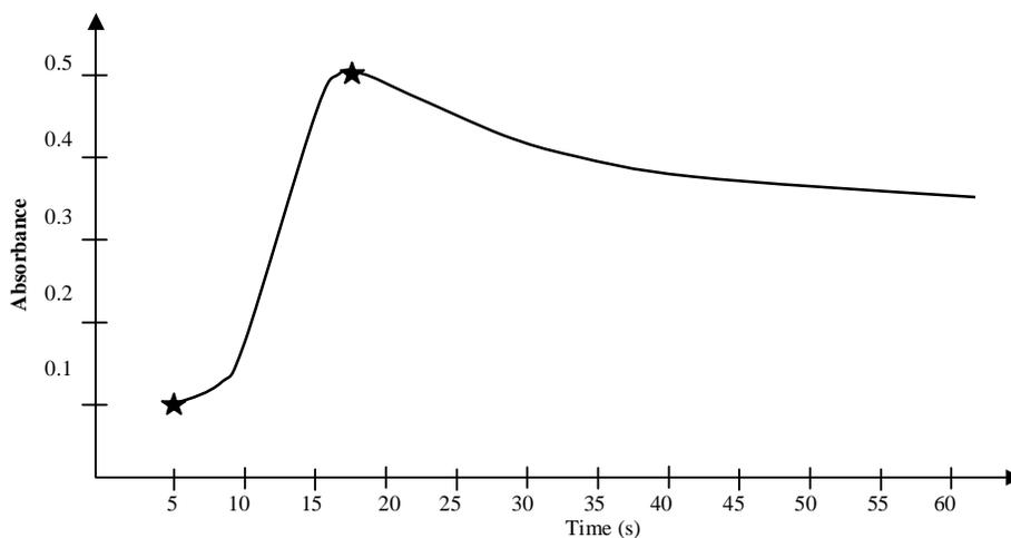
Fig 5: Effect of heating time on the absorbance of the blue complex, formed from 5µg/ml of DHA, 2ml of 0.2% FeCl<sub>3</sub> and 2ml of 0.2% Ferricyanide
