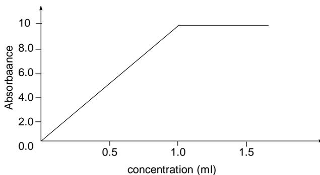
Figure 4: Effect of concentration on the absorbance of formed complex
