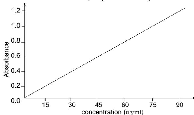
Figure 5: Calibration curve for spectrophotometric method
