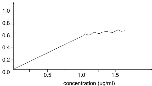
Figure 3: Effect of concentration of thiocyanate on the absorbance of the formed complex
