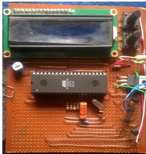
Figure 4: Circuit Construction of Solar Tracker
