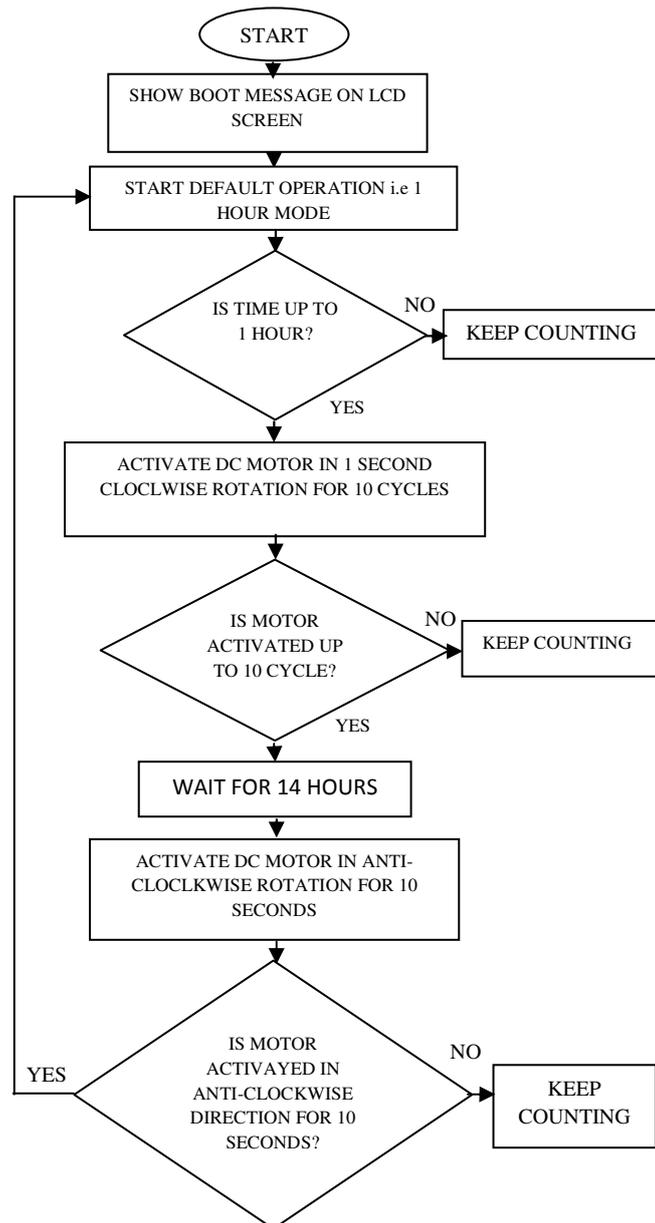
Figure 2: Flowchart of Programmable and Automated Time Dependent Solar Tracker
