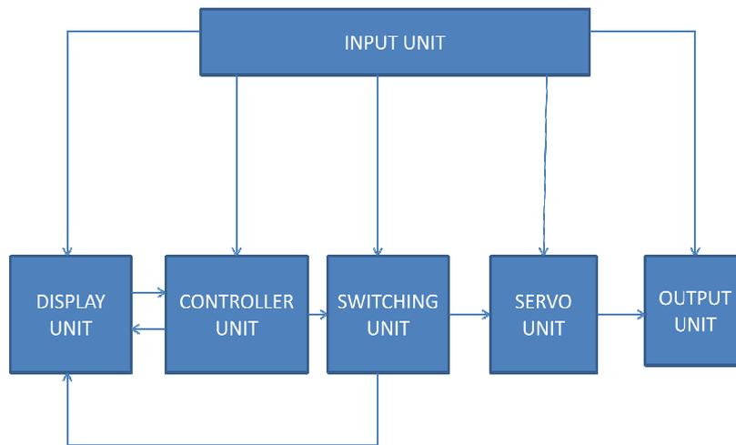
Figure 1: Block diagram of Programmable Automated Time Dependent Solar Tracker
