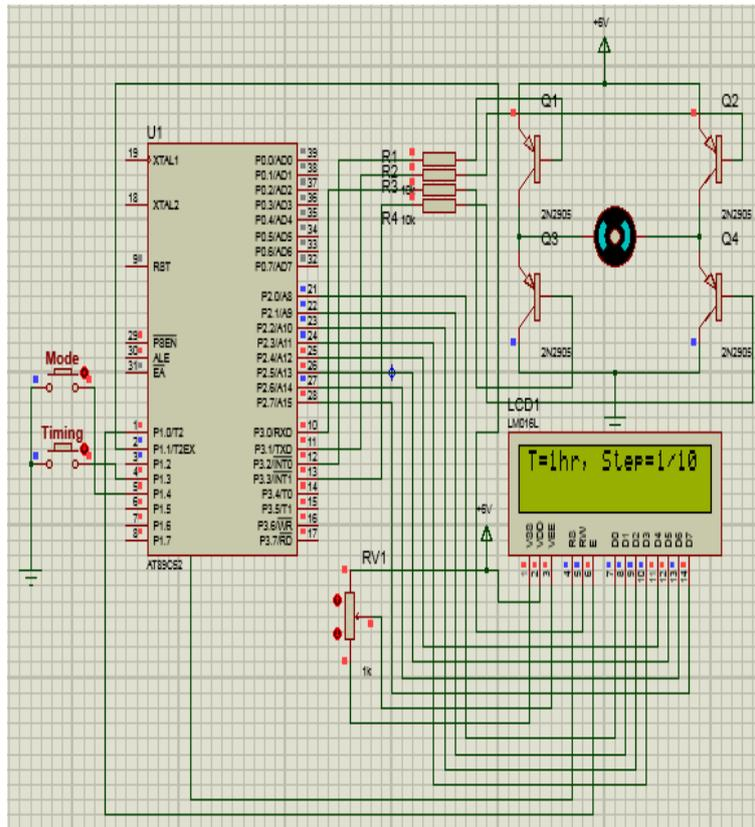
Figure 3: Circuit Diagram of Programmable Automated time Dependent Solar Tracker
