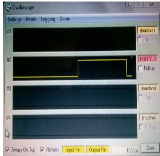
Fig. 5a: Signal Waveform for Clockwise Rotation Fig. 5b: Signal Waveform for Anti-Clockwise Rotation
