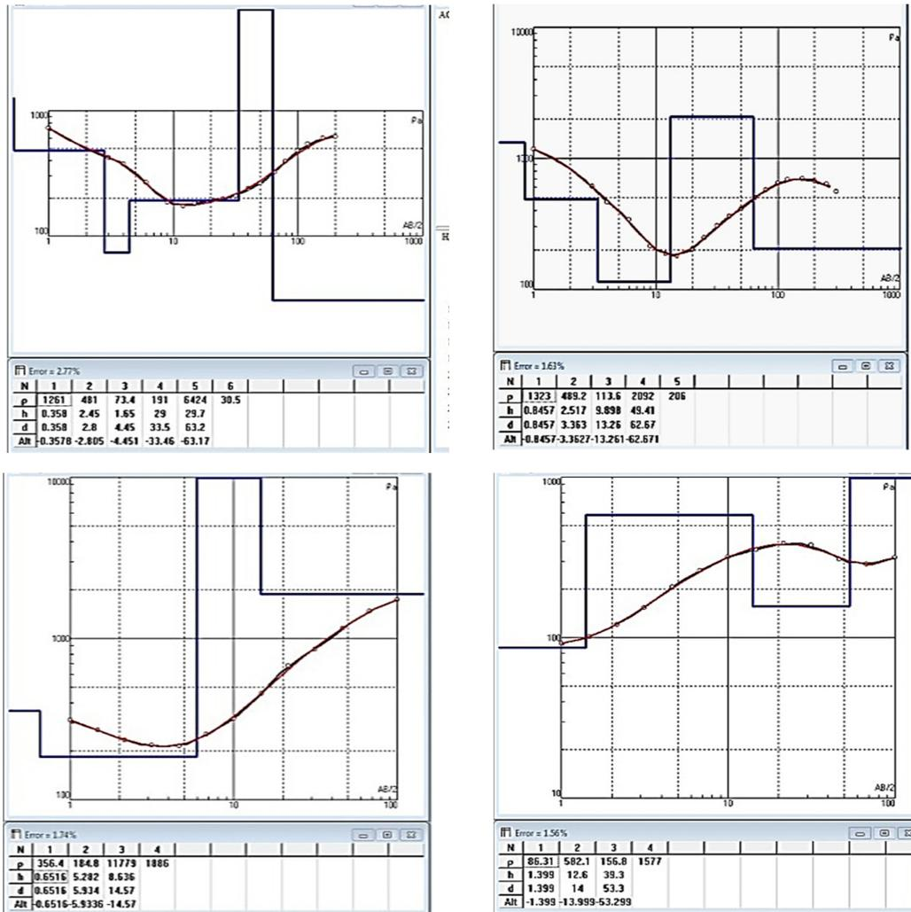
Figure 2. Field sounding curves and interpretative results at Rumuola Pumping station
